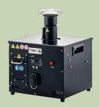
XTIE BIOPARTICLES is an airborne microorganism collection device that utilizes corona discharge to effectively collect and concentrate bacteria and viruses in the air. Using electrostatic attraction, the device has a high collection efficiency of 95% for the 0.1 µm particles.
